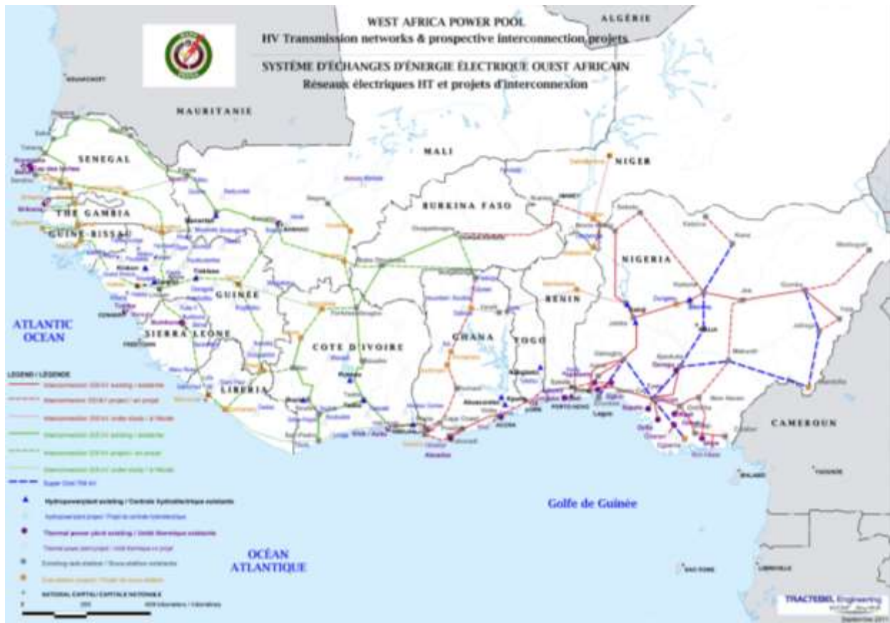
Figure 10: A detailed illustration of existing and proposed interconnections within the WAPP. Image source: (Tractabel Engineering, 2011)
